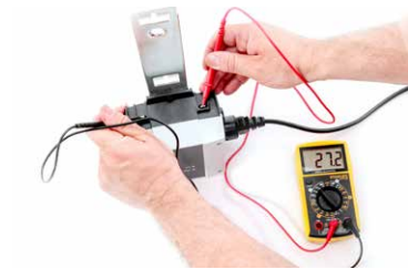
Checking voltage on charger
