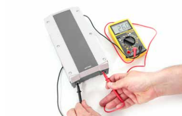
Checking Voltage on battery
