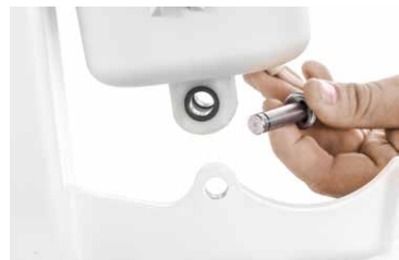
Removing safety clip
