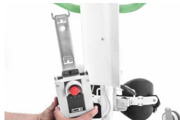
Removing main holder
