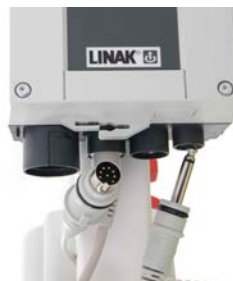
Checking wires connection
