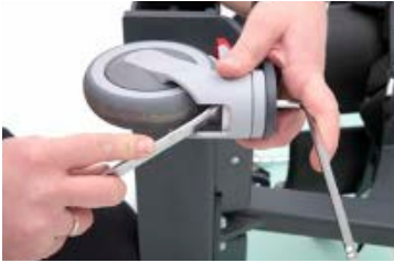
Rear wheels replacement
