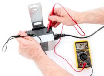
Checking voltage on charger
