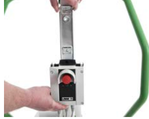
Removing main holder
