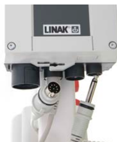
Checking wires connection
