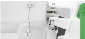
5. Removing safety pin
