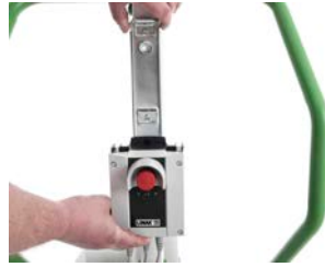
Removing main holder
