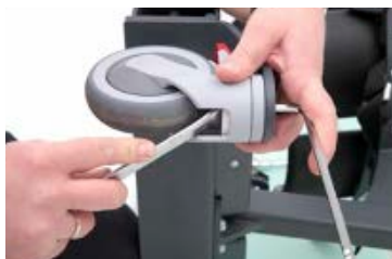
Rear wheels replacement
