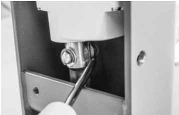
Removing safety ring
