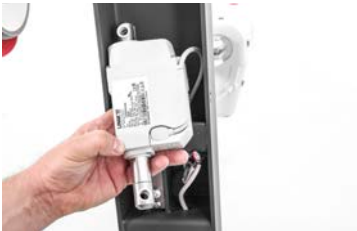
Take out actuator from the frame
