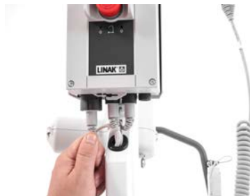
Checking wires connection
