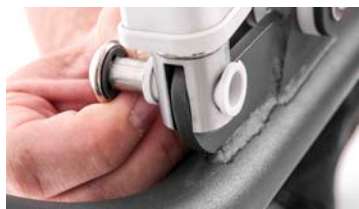
Removing pin(second side)
