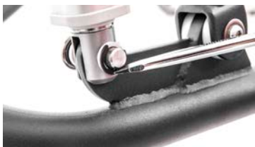
Removing circlip (second side)
