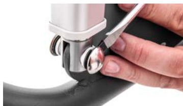
Removing star lock cap(second side)
