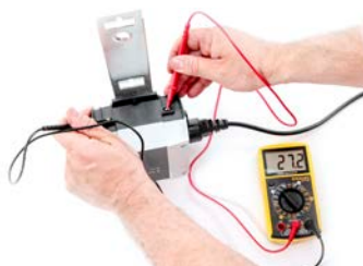
Checking voltage on charger
