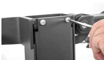
Removing the screws
