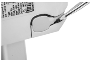
Removing blockade step 1
