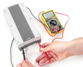
Checking voltage on battery
