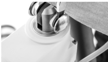
Removing star lock cap
