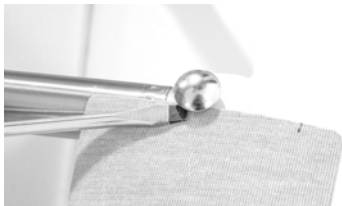
Removing star lock cap
