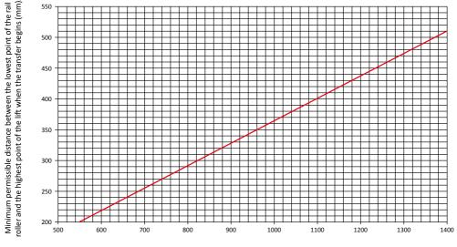
Distance between transfer points (mm). Distances beyond the scope of the diagram are not allowed.
