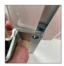
10. Take one of the Screws M10 (8) and add a Washer (7). Assemble the upper hole of the Support Bracket Bottom and the Mounting Plate with an Allen Key 6 mm. Do not tighten the screw fully.
